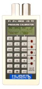
...the pressure calibrator HM38 provides the user with two individual pressure measuring ranges
